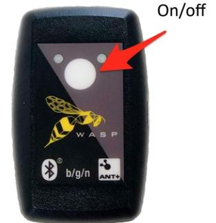
1. Turn off WASP by holding down button for 2-3 seconds. Both LED's will extinguish.
